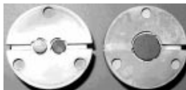
Fig. 4 Photographs of specimen holders for 5\ \text{mm} diameter (left) and 10\ \text{mm} diameter (right), respectively
