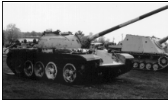
The T-54 was Aleksandr Morozov's last product at the Nizhniy Tagil tank plant. Its revolutionary features included a transverse engine mounting, a powerful 100mm gun, torsion bar suspension, and hemispherical turret. Morozov, at right, carried on a life-long rivalry with Koshkin, the T-34's designer.
