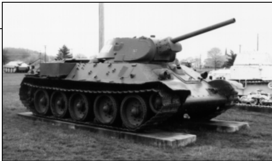
The T-34 Model 1941, seen here at the Ordnance Museum, came as a total shock to German intelligence. Its balanced design combined a relatively large cannon, sloped armor, and a diesel engine on a maneuverable, rugged chassis well adapted to Russian terrain.
