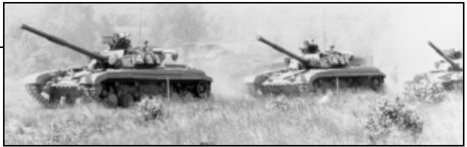
The innovative T-64 was powered by a 5-cylinder flat, opposed-piston engine, used an autoloader in lieu of a fourth crewman, and mounted a 125mm gun that was the largest tank cannon in common use at the time. Reliability suffered with all these innovations.
