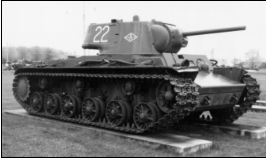
Kotin's KV-1 heavy tank was pressed into production on the basis of very limited employment during the 1939 war with Finland. Unreliable, too heavy, and with no better cannon than the T-34, the KV-1 was an obsolete design.
