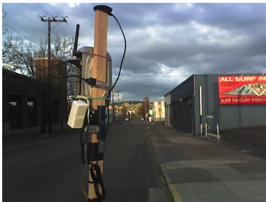
Figure 10: Random-point Connectivity test-rig
