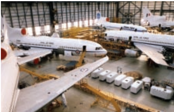
Tristar conversion in progress, No 17 Hangar, Marshalls
