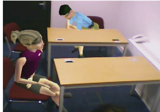
Figure 1. Fully configured view, with the real tables appearing to occlude the virtual avatars.
