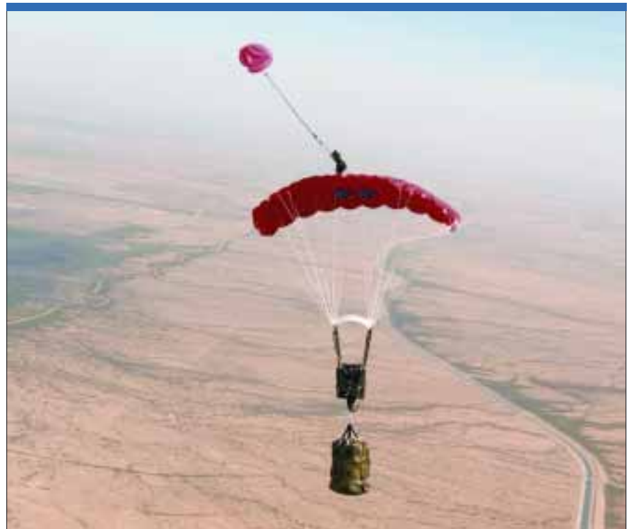
The growing demand for precision delivery from altitude has led to various GPS-guided parafoil systems, one of the leaders in this arena is the Atair Aerospace Onyx series. (Atair).
