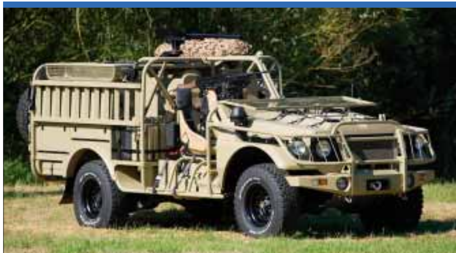
Jankel Armouring has completed the first production version of the Al-Thalab (Fox) long-range patrol vehicle based on a tropicalised Toyota 4 × 4 chassis. (Jankel)
