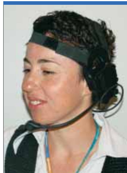
Tadiran Communications has designed a versatile headset for the PNR 500 hand-held radio. Here being modeled by one of the company's media representatives, the unit is available with either a wired or wireless configuration. It features optional wireless PTT unit. (Armada/JK)
