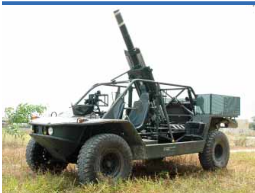
Singapore Technologies Kinetics plans to unveil its 120 mm smoothbore Super Rapid Advanced Mortar System mounted on its 4 × 4 Spider light strike vehicle at Asian Aerospace in February 2006. (Singapore Technologies Kinetics)
