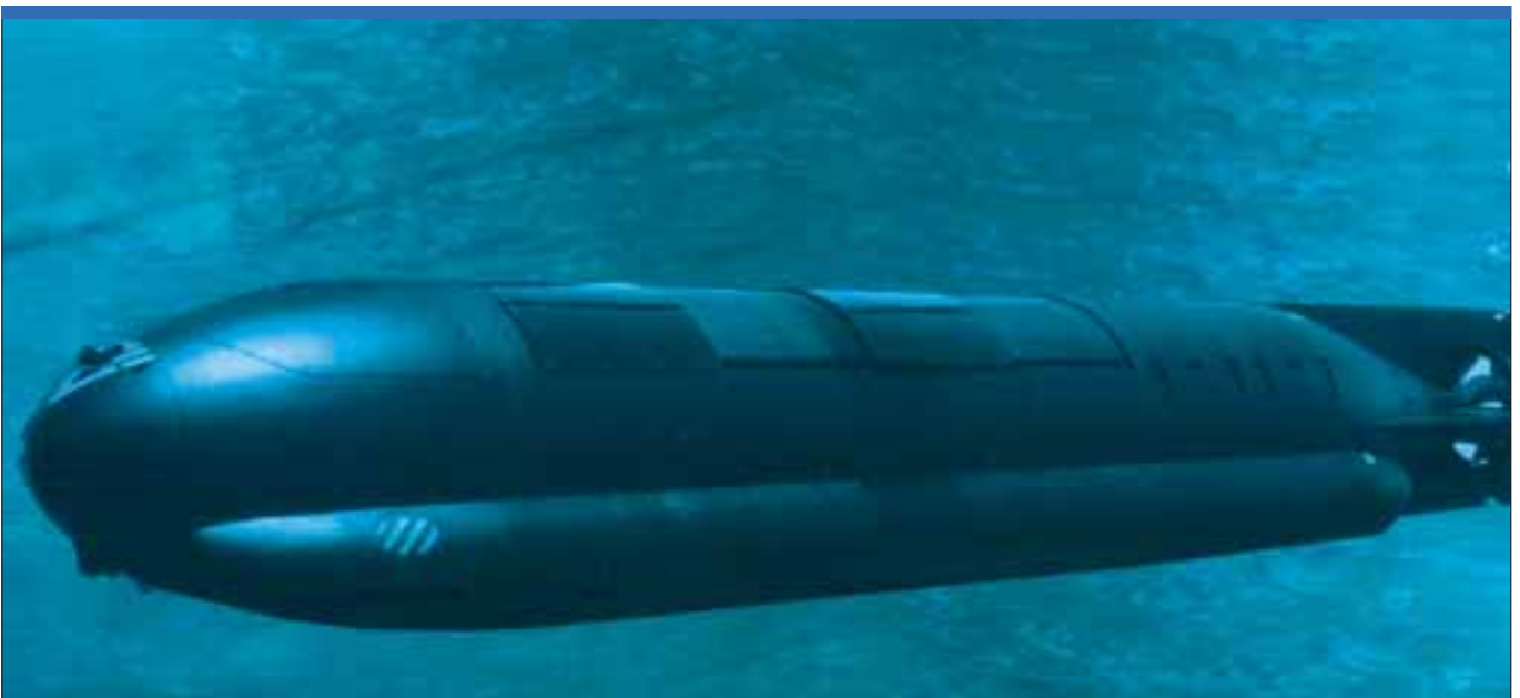
The Class 5 underwater vehicle was exhibited by Emirates Marine Technologies at the 2003 Idex show. An optional fit includes a built-in breathing system providing operators an autonomy of 6 hours. (Emirates Marine Technology)
