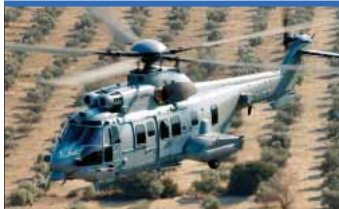
The Eurocopter EC725 'Resco' is a new version of what was originally named the Cougar Mk2+, used by the French Air Force in the combat search and rescue roles. (Eurocopter)
