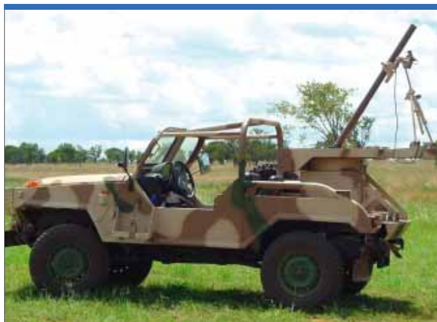
To provide indirect support to special forces and airborne units Denel Ordnance of South Africa is promoting its 4 × 4 Bat Mk II air-droppable light utility vehicle as a platform for the company's 60 mm and 81 mm mortars. (Denel)
