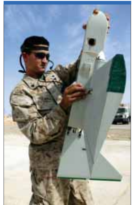
The twin-motor, bungee-launched Dragon Eye was developed by the US Naval Research Laboratory and is produced for the US Marine Corps by Aerovironment. (US Marine Corps)
