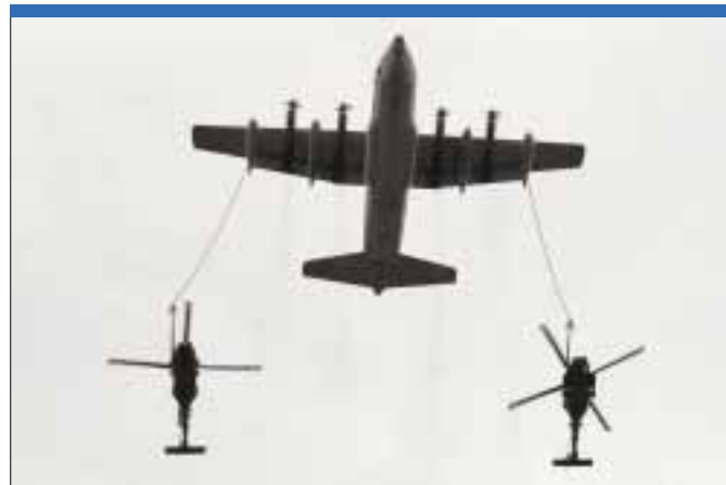
The Lockheed Martin HC-130P/N is the US Air Force's only fixed-wing Combat Search and Rescue aircraft. Its secondary tanker role is shown here, refuelling two HH-60Gs. (US Air Force)
