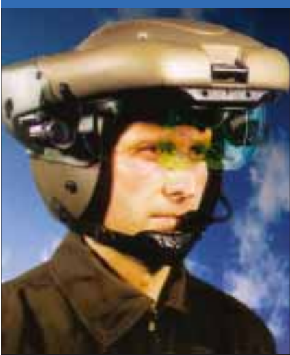
Integrated display helmets like the TopOwl from Thales allow helicopter crews to see the outside world via a flir camera, the Top Owl also displays flight parameters. (Thales)
