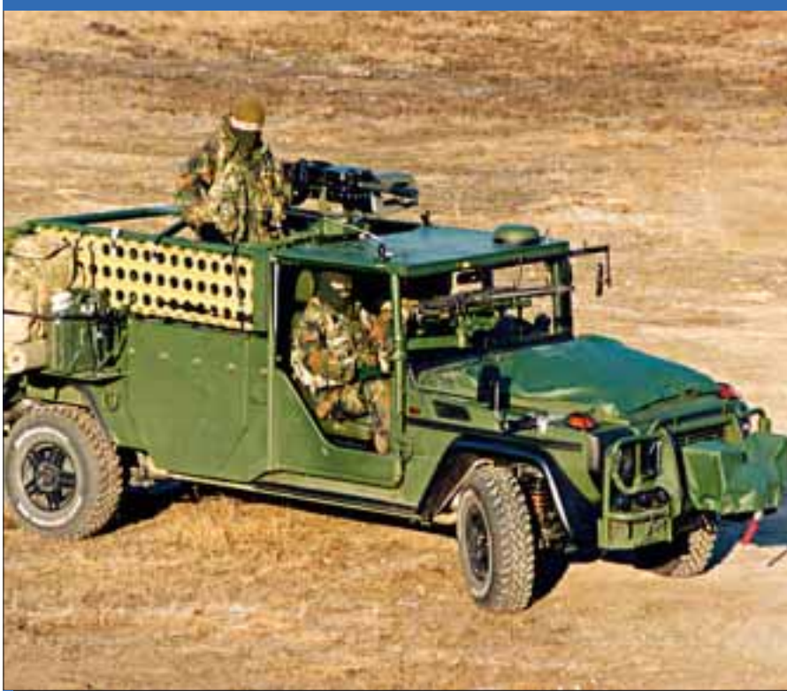
Germany's Rheinmetall Landsysteme has developed the Serval Light Infantry Vehicle (Special Operations) for that country's special forces. The weapon station can be folded to carry the vehicle inside a CH-53 helicopter. (Rheinmetall)
