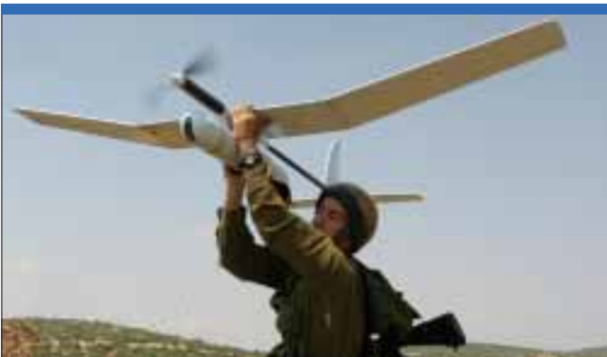
The Elbit Skylark, designed to follow a recent trend in easily delivered drones, is a backpack-carried system for over-the-hill observation. (Elbit)
