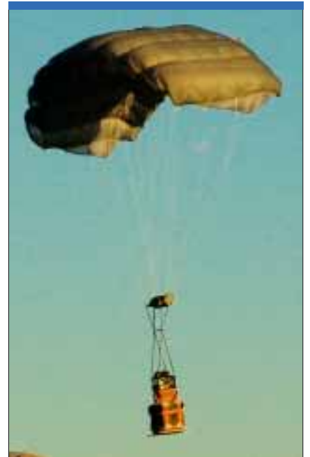
Dutch Space and the Netherlands' National Aerospace Laboratory (NLR) are developing the GPS-guided Spades (Small Parafoil Autonomous Delivery System), which is shown here during tests. (Dutch Space)
