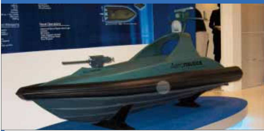
After Rafael had developed the unmanned Protector with Aeronautics, the latter firm presented its own iteration, the six-tonne SeaStar at the 2005 Paris Air Show. It can be armed with a variety of stabilised weapons, perform electronic intelligence and electronic countermeasure missions and reach 45 knots. (Armada/EHB)
