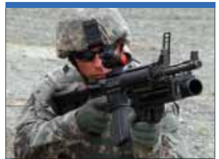
A Heckler & Koch 40 mm XM320 Grenade Launcher Module attached to a 5.56 mm M4 carbine. The US Army has selected the XM320 to replace its ageing M203 launchers. (US Army)
