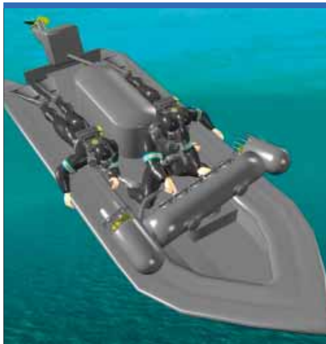
An interesting device is the hybrid Subskimmer, basically a Zodiac-type boat that is deflated when the diving point is reached. Propulsion is then switched from piston-engine to electric. (Armada archive)
