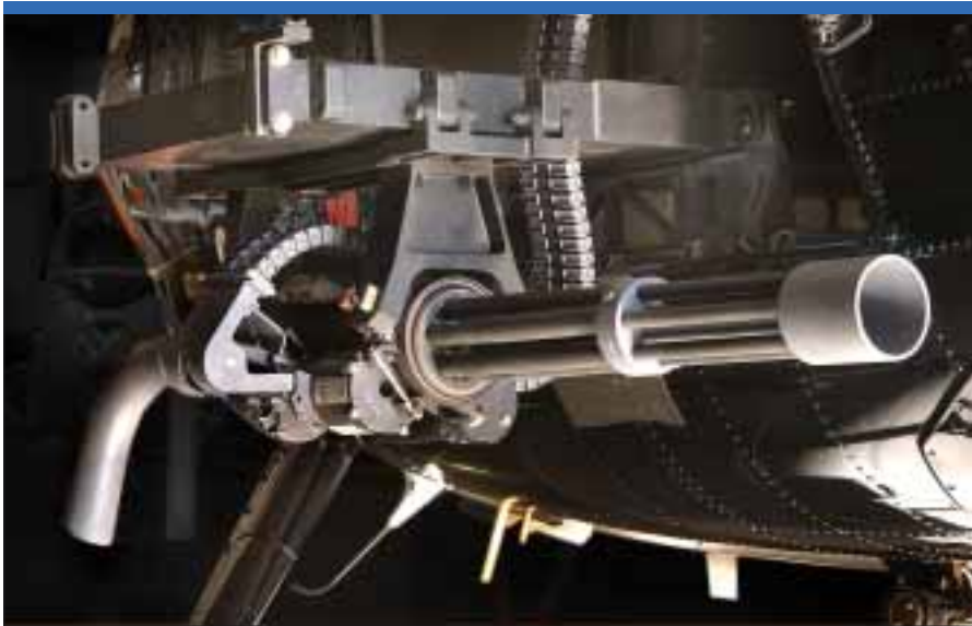
There apparently is a marked (or renewed?) interest for lighter and more flexible helicopter armament as war against terrorism intensifies. Indeed, stopping a 4 x 4 Toyota with a Hellfire might be spectacular on television, but the Minigun revamped by Dillon Aero as the M134D for example, is definitely up to the job. (Dillon Aero)
