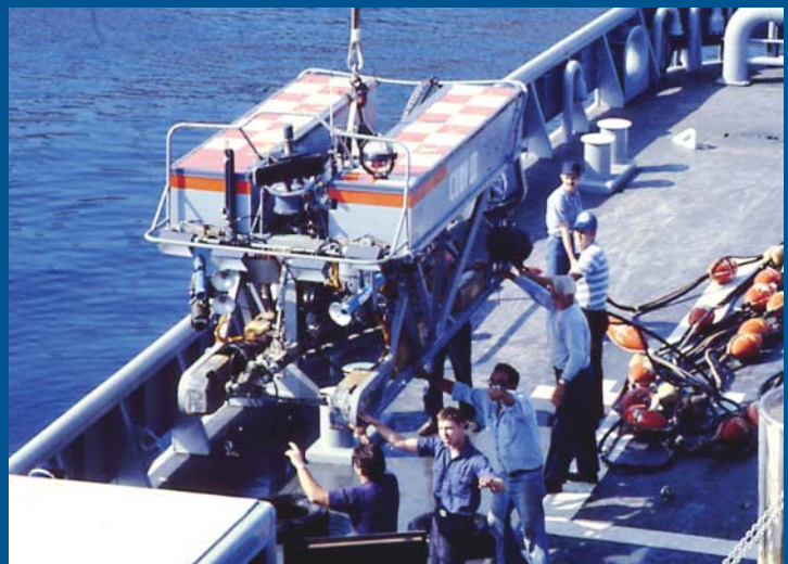
ROV CURV III being loaded over side. CURV III can dive to a depth of 6,000 meters.
