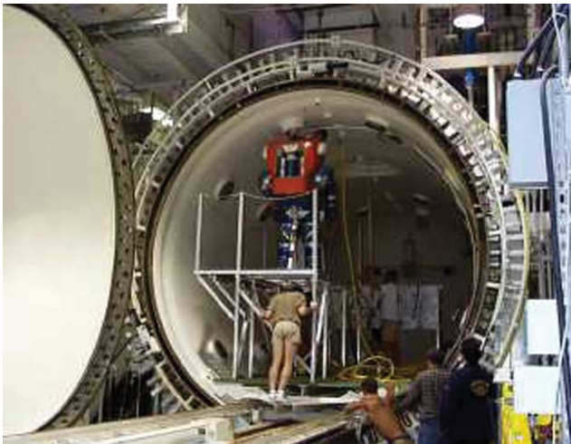
Ocean Simulation Facility, 55,000 gallon wet pot.
