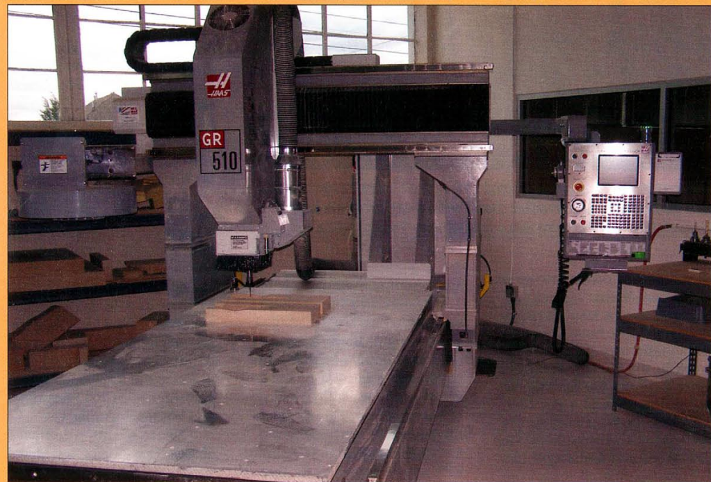
One of the more unusual machines at the MotoCzysz plant is a computer-controlled mold-making machine. It carves hard, dense foam into computer-generated shapes to allow for rapid prototyping, and finished production of composite pieces. Composite construction has its own dedicated room of about 1000 square feet.
