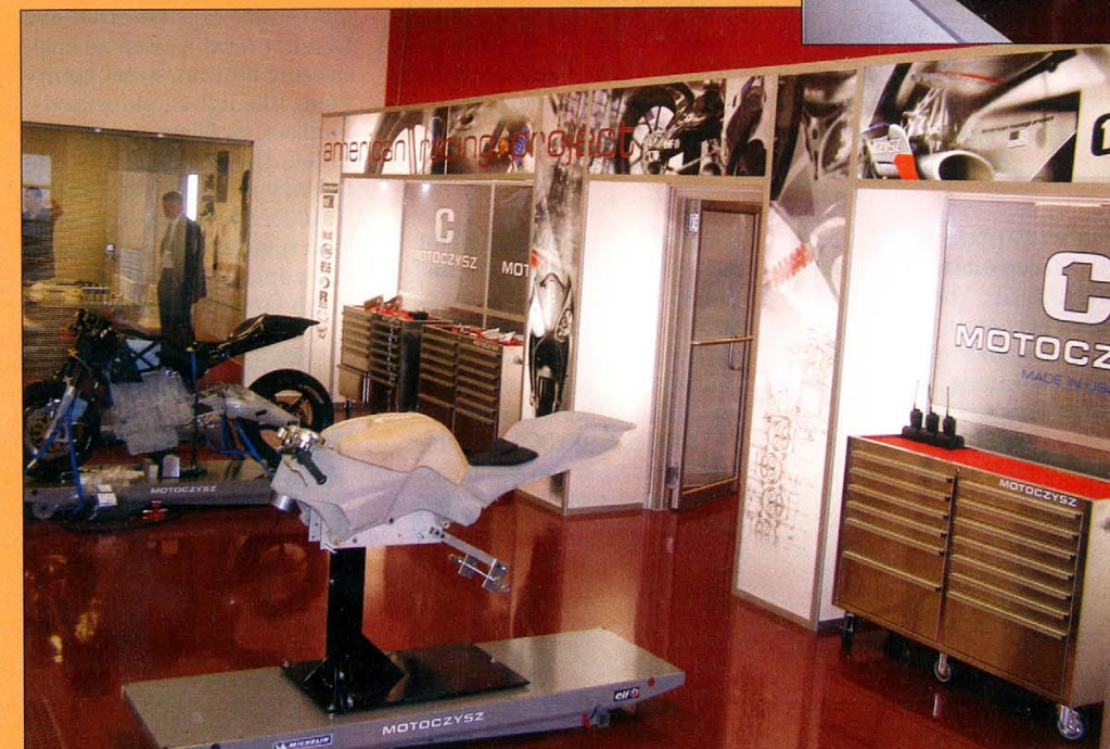
Part workshop, part showcase, part investor relations: The assembly room for the new C1. In the foreground is a frame made of rapid prototype epoxy, in the background is an actual chassis with a rapid prototype engine, behind the glass in the far background is a meeting room with an actual angel investor inside.
