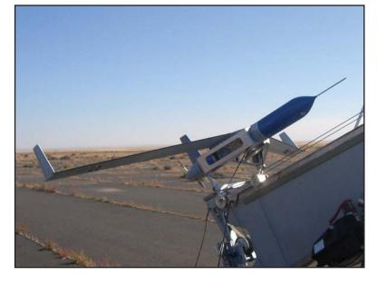
**GeoRanger™** is designed and built for sophisticated remote sensing missions using advanced electronic instruments. GeoRanger is delivered with the customized payload capacity for a proprietary cesium magnetometer, plus a data collection expansion board for the modular avionics bay slot. GeoRanger is exclusively provided to Fugro for their geophysical survey business, and Fugro supplies and integrates the magnetometer and data collection electronics.
