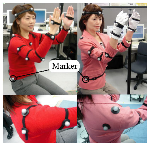
Figure 6: Marker positions on the master (right) and android (left)
