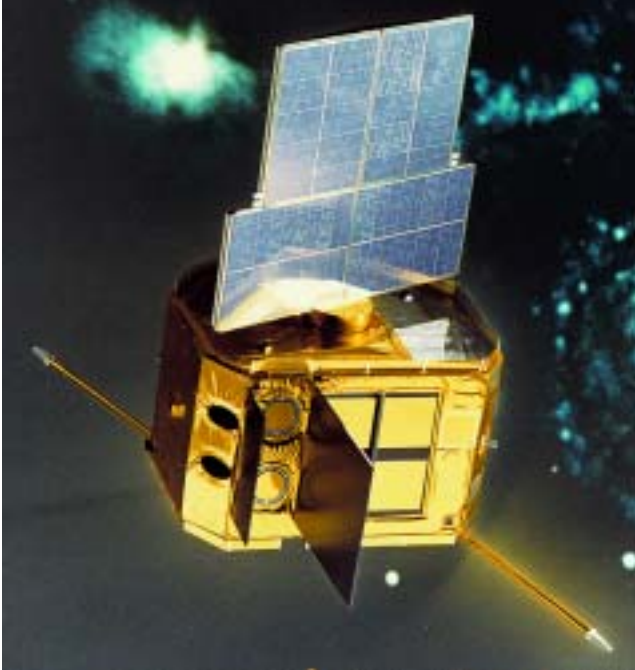
Exosat in operating configuration. On the front, from left to right, are two startrackers, the two low-energy imaging telescopes and the four quadrants of the medium-energy instrument. The gas scintillation proportional counter is visible to the right of the medium energy instrument.
