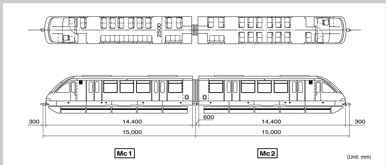
Figure 5 HSST-100L Vehicle Design
