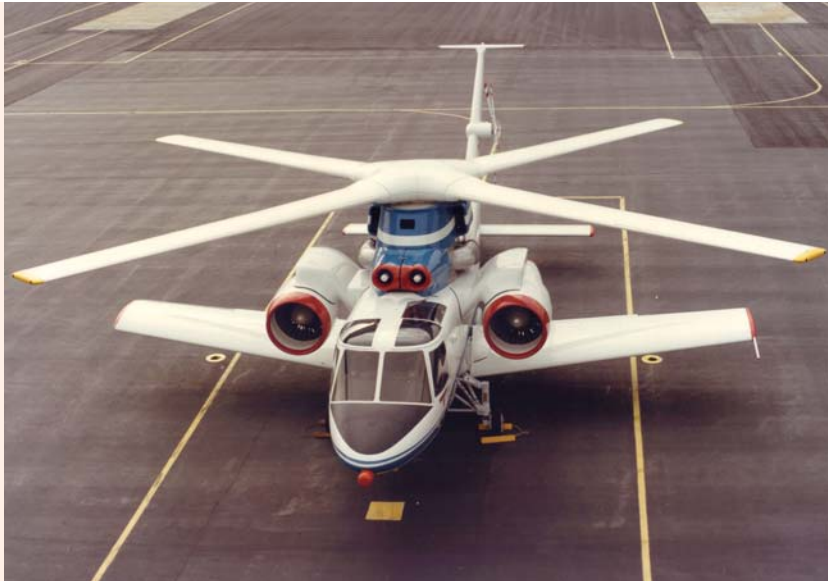
Although the X-Wing's circulation control rotor system was ground tested extensively, it was quite a challenging concept. Sikorsky's S-72X is shown here with a flightworthy and operating X-Wing rotor, but it never left the ground.
