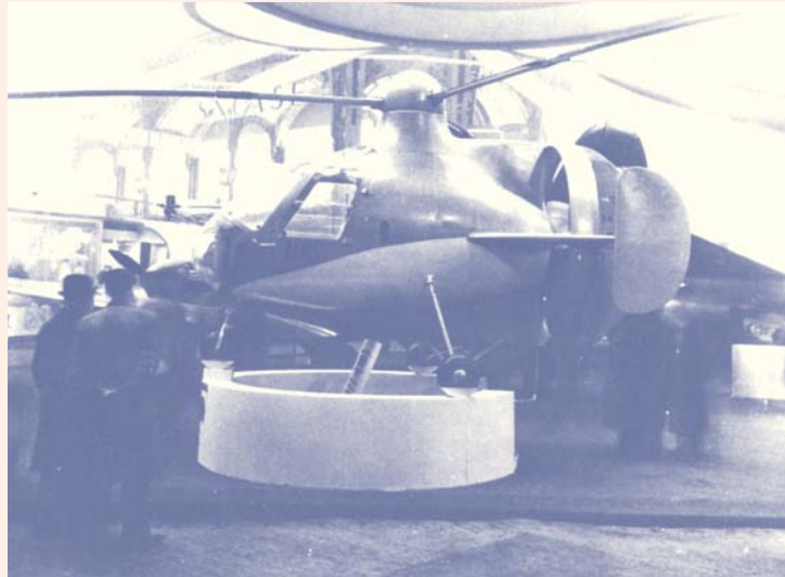
The original Sud-Ouest Ariel was intended to use tip-jets for vertical and hover flight and a pusher propeller for high-speed forward flight. Unfortunately, it never progressed beyond limited hover flights.
