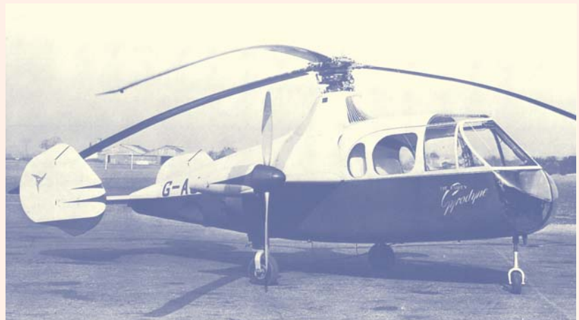
The Fairey Gyrodyne - with a three-bladed rotor and a tractor propeller - was the first compound helicopter to take flight in the United Kingdom.
