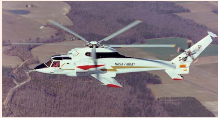
The Sikorsky S-72 Rotor Systems Research Aircraft (RSRA) had the unique ability to fly as a pure helicopter, a compound helicopter, or as a fixed-wing aircraft.
