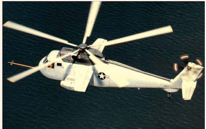
Sikorsky's heavily-modified Sea King, the S-61F, possessed a number of drag-reduction features designed to permit higher speeds.
