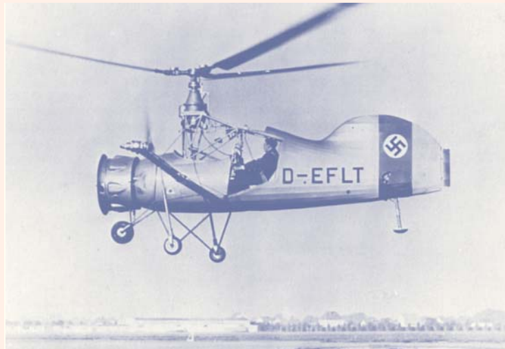
The Flettner Fl 185 used two propellers mounted on outriggers. They were used for anti-torque and for forward thrust.
