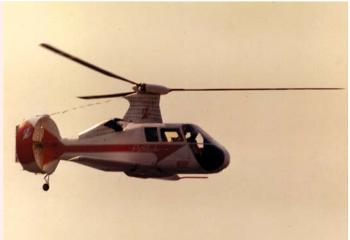
Piasecki pioneered the Ring-Tail on its 16H-1 Pathfinder as a means of auxiliary propulsion and anti-torque control.
