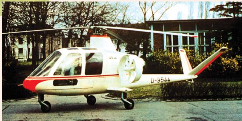
The VFW H3 was to have used a set of ducted propellers for high-speed flight. Its jump takeoff performance earned it the nickname "Sprinter."
