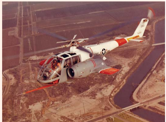
The diminutive Lockheed XH-51A Compound used small wings and a J60 turbojet to attain an unofficial rotary-wing speed record of 302.6 mph in 1967.
