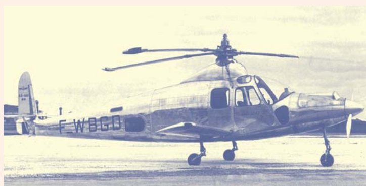
Using high-pressure exhaust outlets and a rudder to control yaw, the Sud-Ouest Farfadet was a very stable and controllable aircraft to fly.
