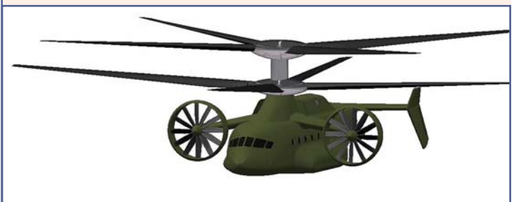
Sikorsky's X2 rotor technology could be applied to a wide range of future platforms, such as the high-speed heavy lifter being studied for the Army.
