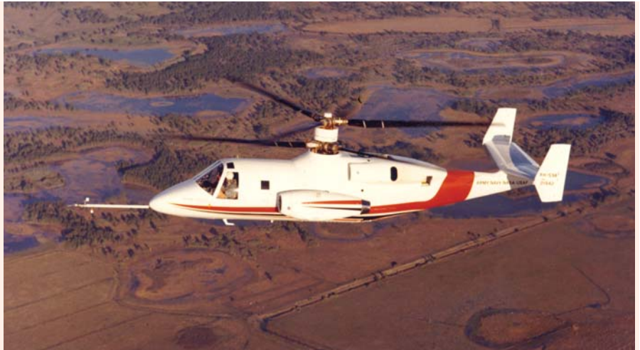
The Sikorsky S-69 exploited the inherent advantages of the Advancing Blade Concept (ABC) by eliminating retreating blade stall.
