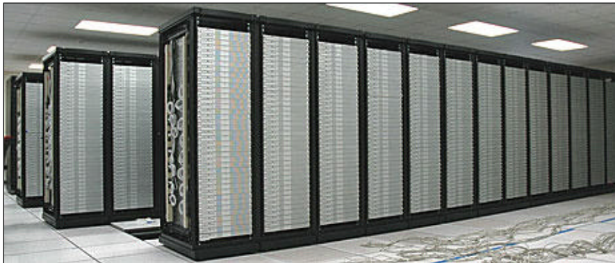
One of the world's largest and most powerful computers: a supercluster of 1,566 64-bit, dual-processor Apple Xserve G5 servers.
