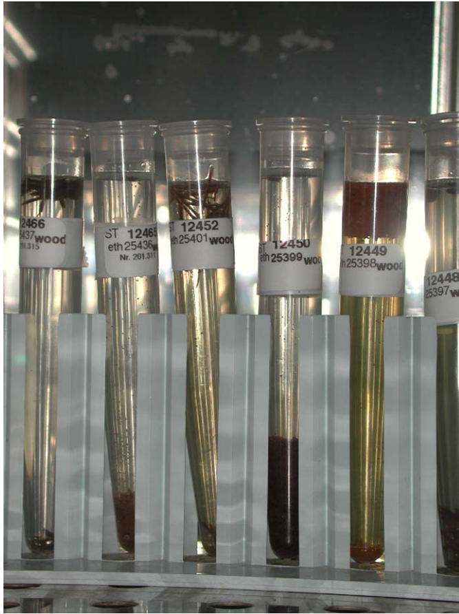
Fig. 4. The standard acid–alkali–acid procedure of cleaning organic material involves a sequence of washes in acid, base and acid to remove contamination by carbonates and humic acids.
