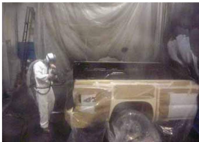
Spraying base coat with protective equipment.
