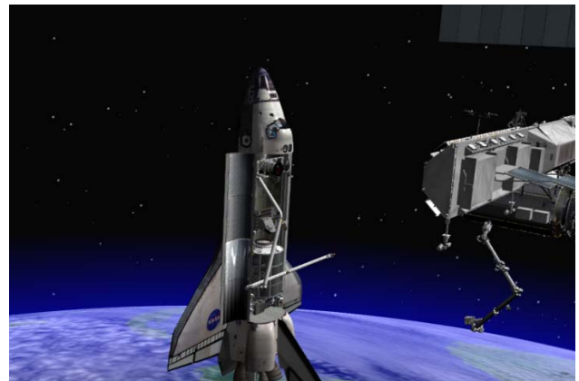
Artist's rendering of Discovery undocking from ISS with the OBSS in the hand-off position.
