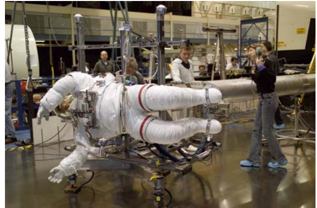
Astronaut Piers J. Sellers, wearing a training version of the extravehicular mobility unit spacesuit, participates in a simulation. He is anchored on the end of the training version of the space shuttle remote manipulator system (RMS) robotic arm in the Space Vehicle Mockup Facility at Johnson Space Center. Lora Bailey (right), manager, JSC engineering tile repair, assisted Sellers. Astronaut Michael E. Fossum (center), mission specialist, also participated in the test.
