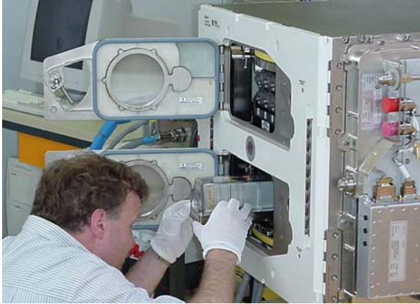
ESA astronaut Reinhold Ewald inserts an experiment container into the EMCS Engineering Model.
