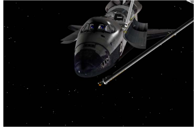
Artist's rendering of the OBSS inspection of Discovery's nose cap heat shield.
