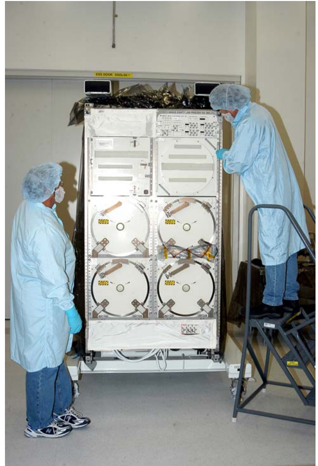
Technicians inspect the Minus Eighty Lab Freezer for ISS (MELFI) at NASA's Kennedy Space Center.
