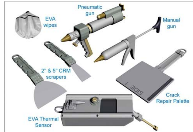
Engineering models show the various RCC repair tools the crew will use during the test.
