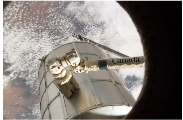
The Canadarm2 grasps the Italian-built MPLM Raffaello to place it back in Discovery's cargo bay during STS-114. The Earth forms the background.
