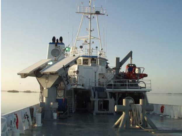
NASA X-band radar on the fantail of "Freedom Star" - one of two solid rocket booster recovery ships
