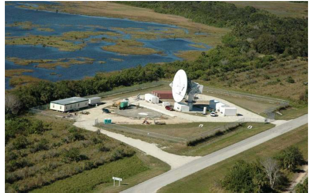
The 50-foot, C-band radar located at the NDR-1 site north of the Kennedy Space Center
