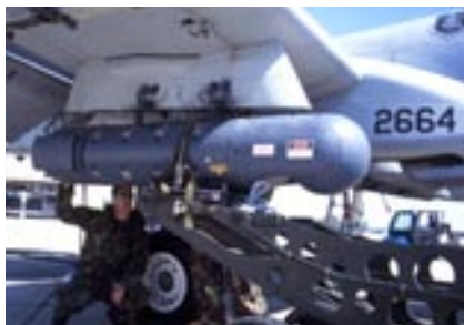
At left, airmen complete the installation of the pod while, at right, the A-10 taxis onto the apron. USAF plans to further upgrade its Warthog fleet to the precision engagement A-10C configuration. These "Hogs," now under development, will have digital cockpits and a wider weapons selection.
