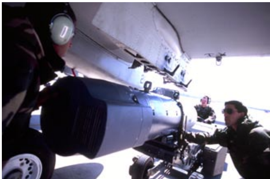
Airmen of the 23rd FG at Pope install a Litening II pod. Above, SrA. Mark Fesperman drives a "Jammer," while SrA. Daniel Galloway (kneeling) and A1C Robert Perry work the pod into position. At right, Fesperman and Galloway raise the pod onto the wing's hardpoint.
