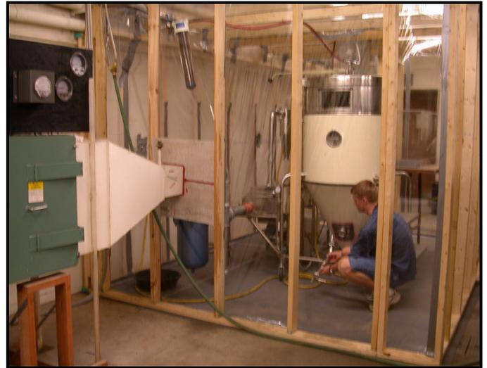
Fig. 14 Photograph of the Spray Drying System Showing the Chamber and HEPA Filtration System.
