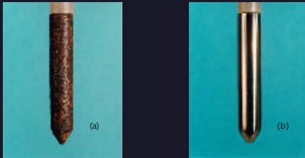
Diesel fuels showing (a) insufficient and (b) suitable anti-corrosion performance
