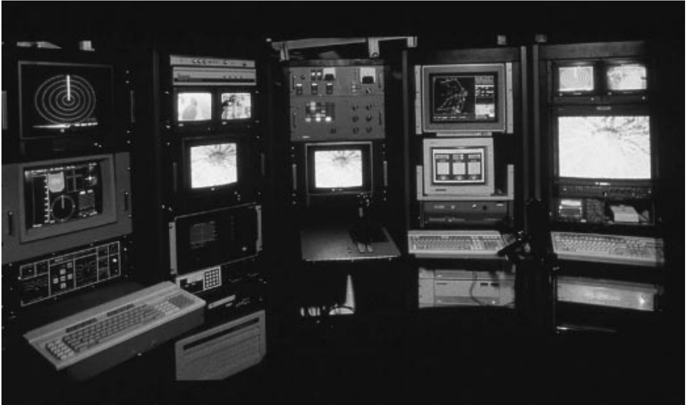
The science control room aboard the R/V Point Lobos contains monitors and control panels used to navigate Ventura and manipulate instruments while scientists and pilots view video images and displays of oceanographic data.
