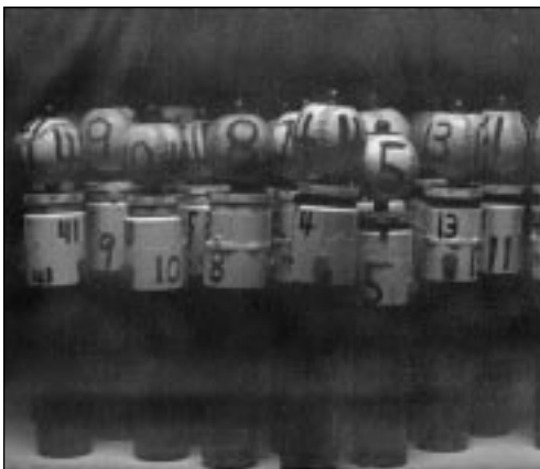
The manipulator arm on Ventana can grab a softball on one of these push-core devices, then push the tube into the seafloor to collect sediments.
