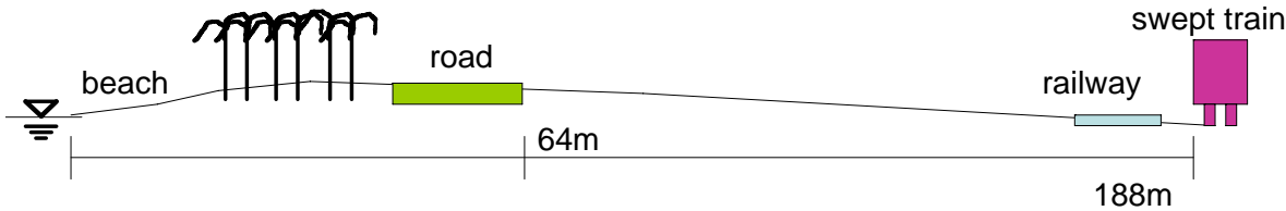
Figure 3 Cross section of the damaged area, Kahawa, where the train was washed away
