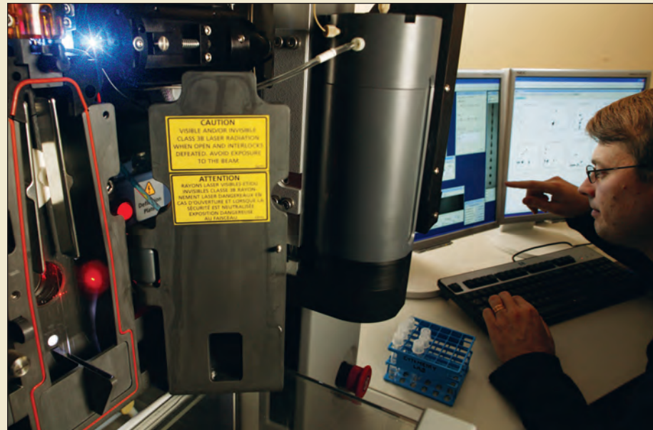
Creighton's Patrick Swanson, Ph.D., associate professor of medical microbiology and immunology, works with the new BD FACSAria flow cytometer, which can sort cells 10 times faster than any previous instrument.
