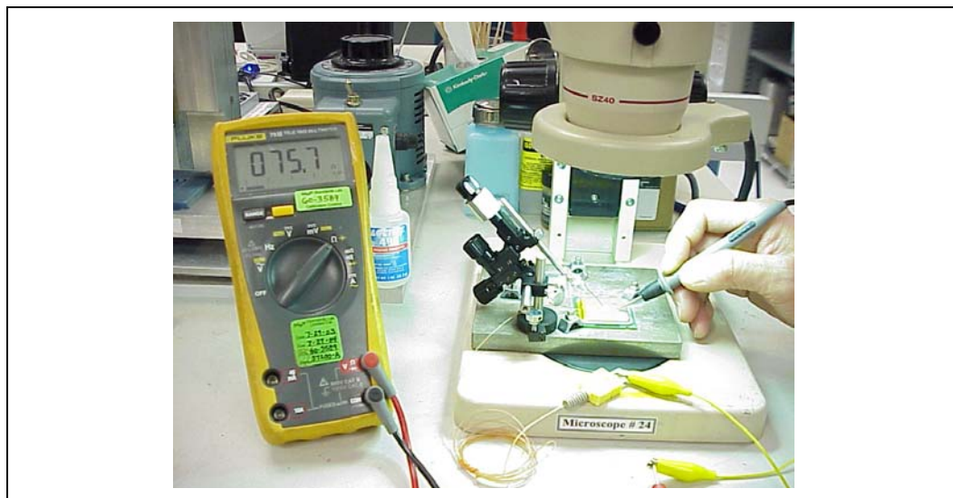
Figure 36. Measuring Resistance between Thermocouple and IHS
