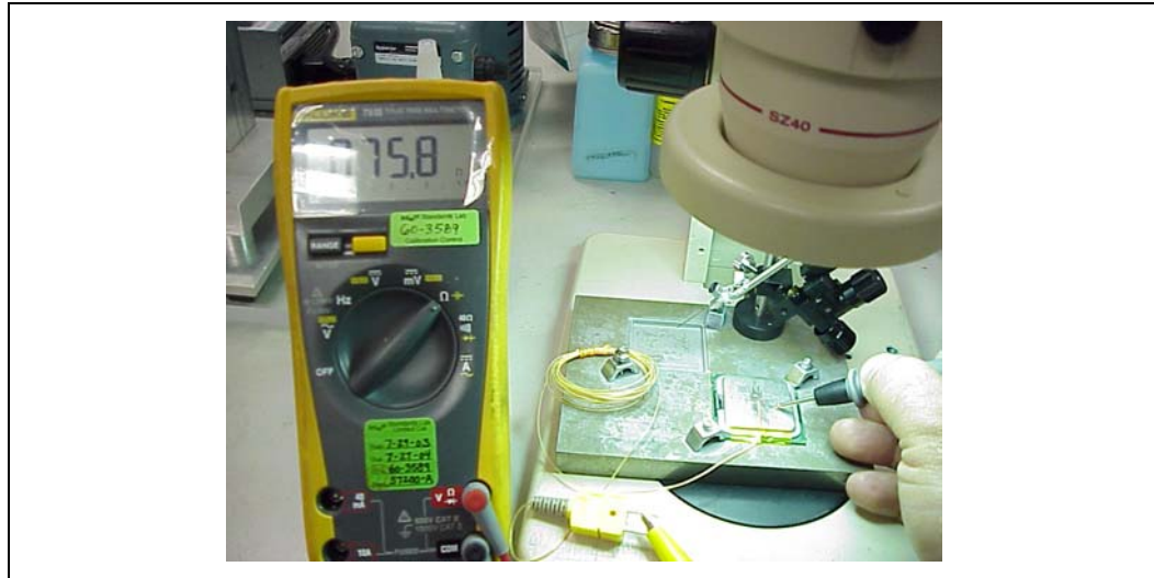
Figure 37. Applying the Adhesive on the Thermocouple Bead
