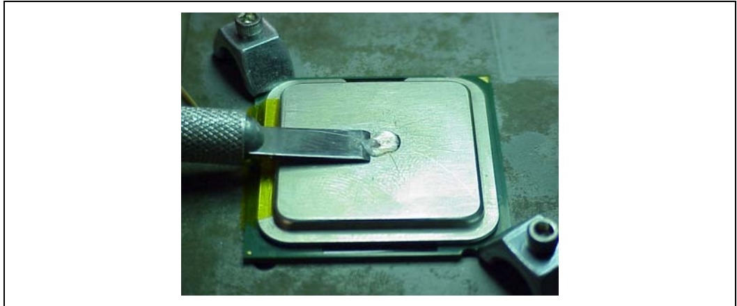
Figure 39. Removing Excess Adhesive from IHS
