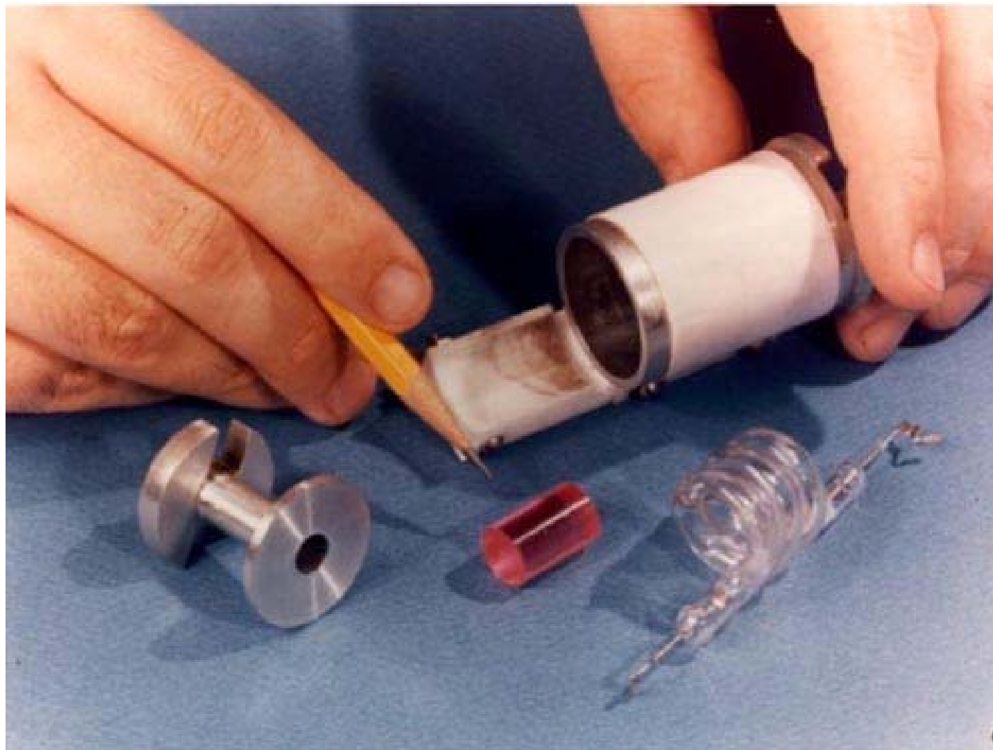
First ruby laser, disassembled
