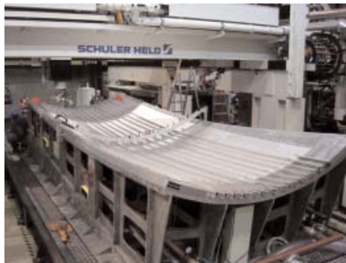
XXL laser-beam welding plant with welding shell.
