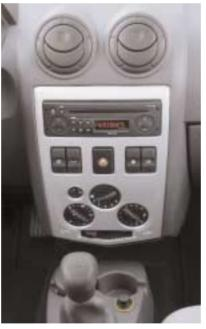
It is very compact, freeing up space in the cockpit. The upper and lower vents ensure optimum distribution of air flows.
