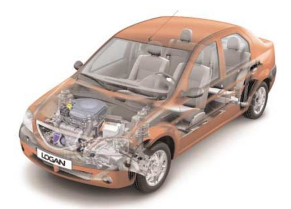
In the event of a side impact, the central pillar protects the pelvis, complementing the lateral resistance provided by the seats and door padding. Rear impacts were also the focus of attention. The fuel tank is located under the floorpan, away from the rear suspension, so there is less chance of it being pierced by the underbody or suspension components. A cross-member in the back of the rear bench seat restricts the danger of objects in the boot entering the cabin.
