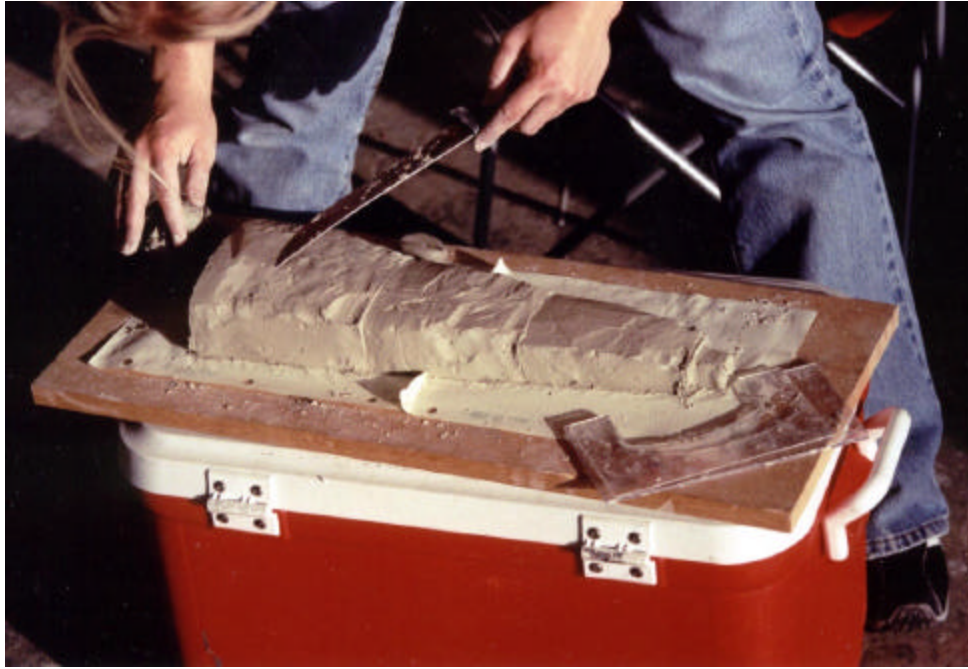
Figure 3.7.: Forming the mold using modeling clay and templates
