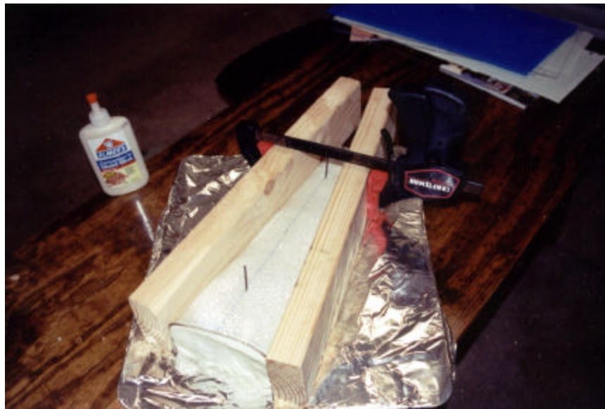
Figure 3.9: The thermoformed acrylic was clamped and allowed to cool
