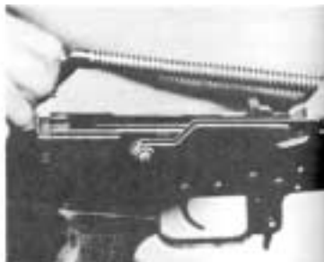
Removing the recoil spring assembly of the BB.
