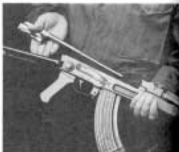
Removing the bolt carrier assembly.
