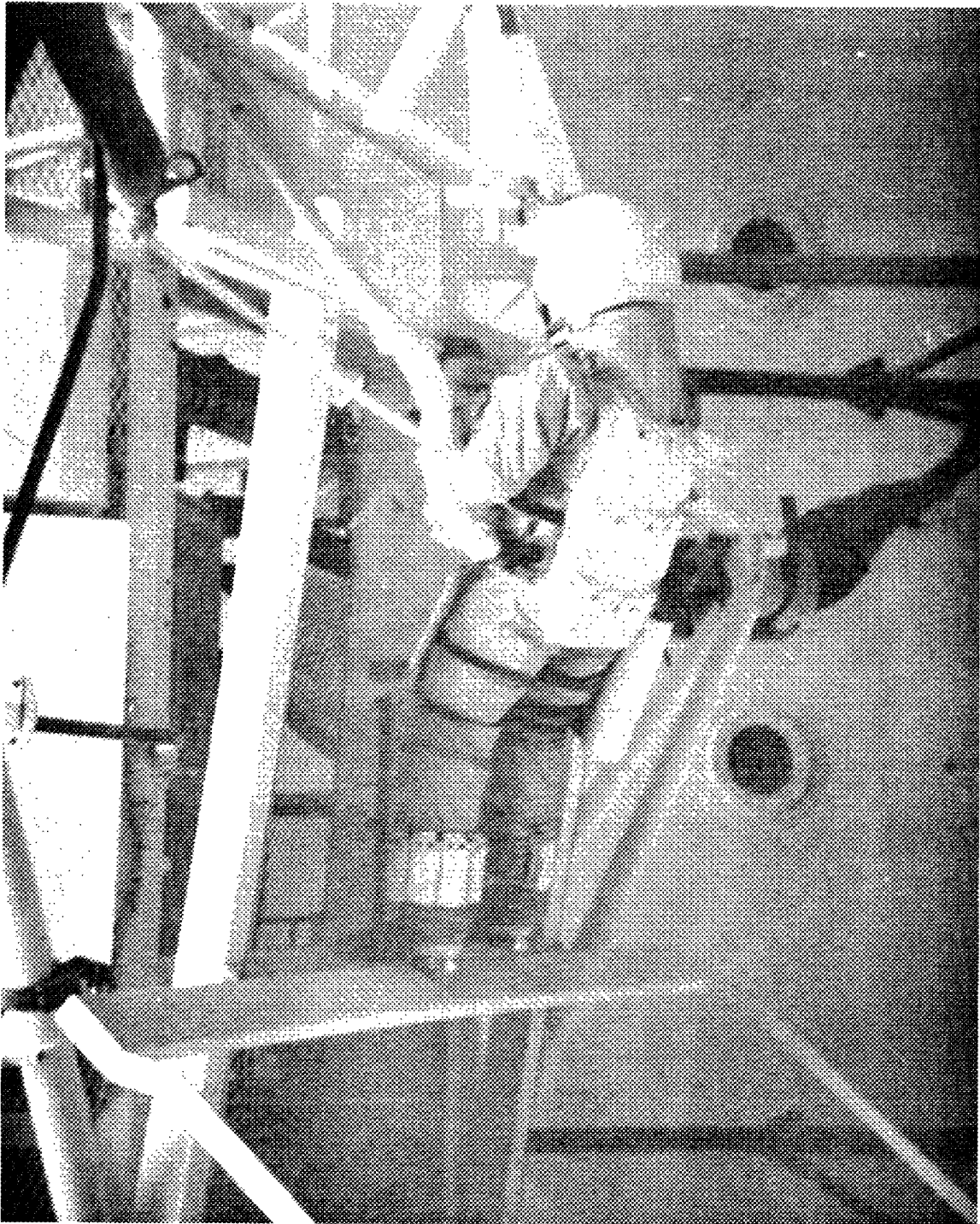
Figure III. In the final position, the crewman transfers his feet to force the solar panel slide bar along the support structure and completes the deployment. The center workstation is now accessible for film retrieval.
