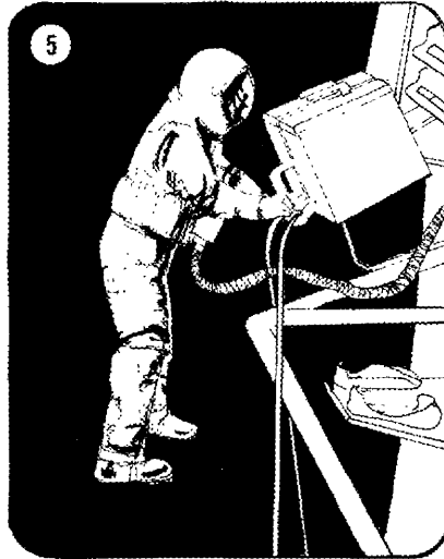
Figure 67. EVA Film Retrieval Procedure
