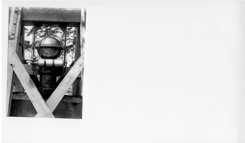
The rocket engine designed by Arthur Rudolph was the heart of the A-1 rocket, built by the Army at its experimental station in Kummersdorf. This photograph of the engine on a test stand was taken in 1934. Deutsches Museum
