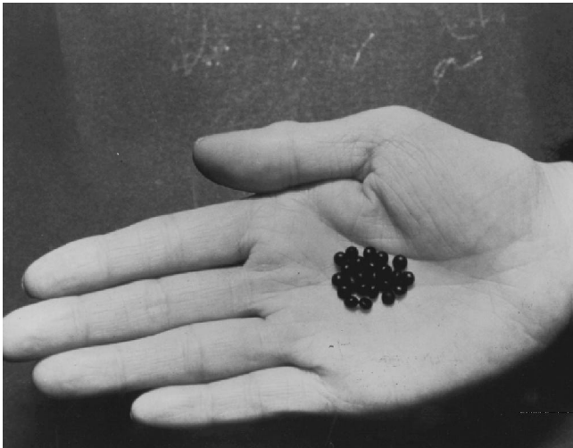
Help from nature. U.S. Bureau of Mines scientists developed these tiny, porous beads made from peat moss and polymers to extract metal ions from waste water. Photo credit - USBM.
