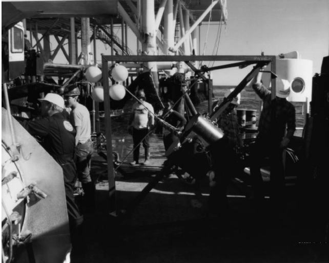
MMS scientists place strong motion instruments beneath the sea floor in the Santa Barbara Channel to better understand the effects of earthquakes on offshore structures. Photo credit - MMS.
