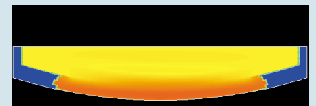
Prediction of neck down, velocity and temperature in optical fiber drenching. Significant draw-down ratios, coupled flow of glass and helium, along with spectral radiation, characterize this process.
