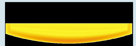
Coupled plunger motion and glass shape in a mold for making TV panels.
