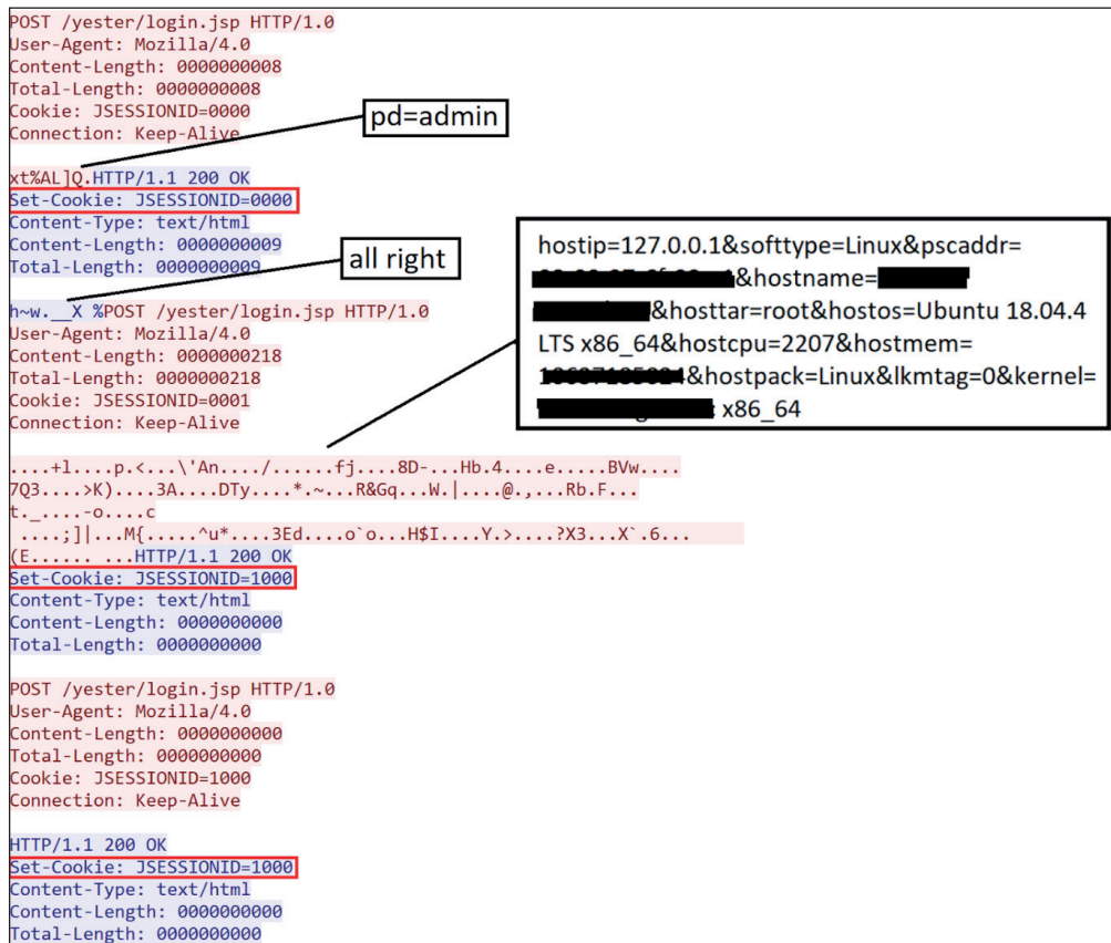
Figure 9: RedXOR communication with C2.
