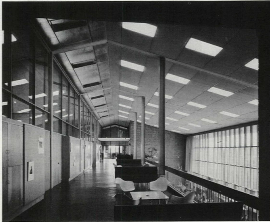
North-facing meeting rooms at left of the upper-level balcony lounge (above) borrow south light through partition glazing.
