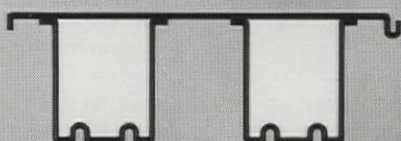
SECTION M2-7.5 CEL-BEAM DEPTH 7 1/2"
