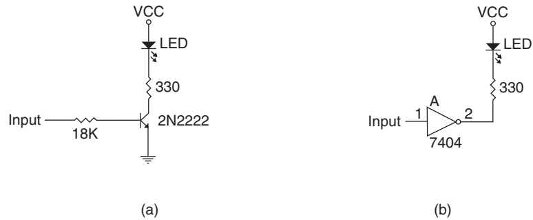
FIGURE 11–8 Interfacing an LED: (a) using a transistor and (b) using an inverter.
