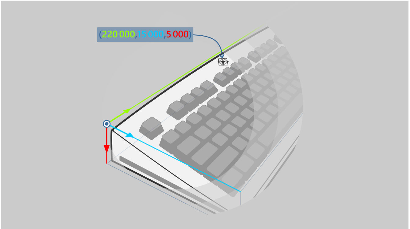
Figure 24.5: Keyboard branding lamp under the logo. Position of lamp relative to the bounding box (described above) labeled in \mu\text{m} .
