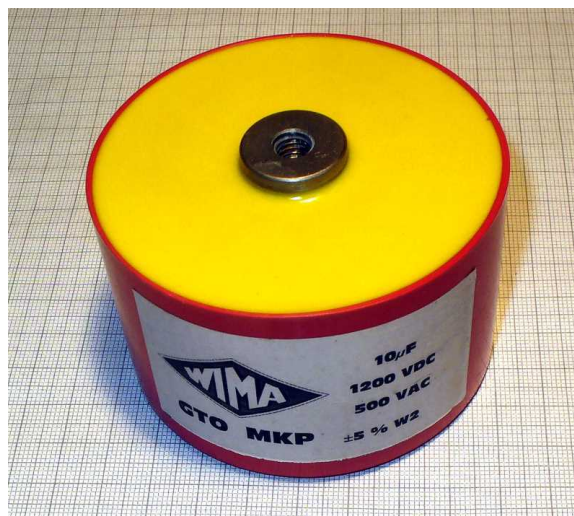
Figure 53 Heavy-duty snubber capacitor with screw terminals
