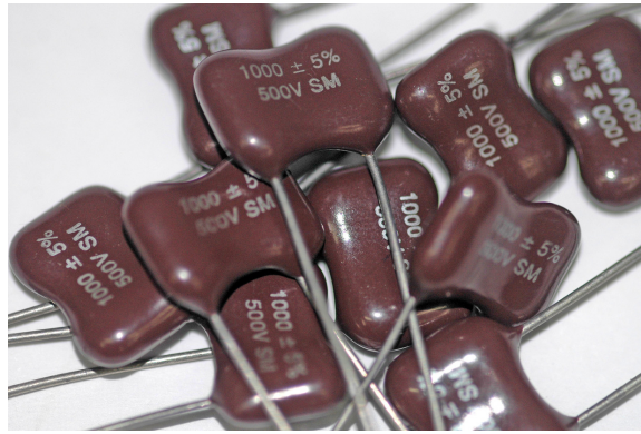
Figure 71 Some 1nF × 500VDC rated silver mica capacitors
