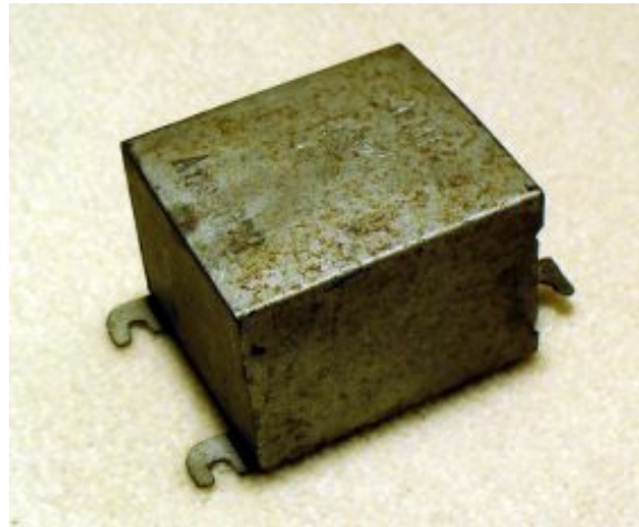
Figure 39 Stacked paper capacitor (Block capacitor) from 1923 for noise decoupling (blocking) in telegraph lines
