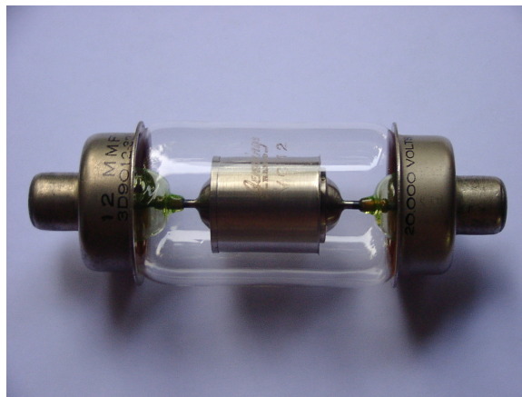
Figure 72 Vacuum capacitor with uranium glass encapsulation
