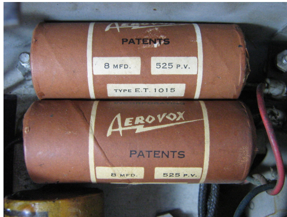
Figure 42 Two 8 \mu\text{F} , 525 V wound wet aluminum electrolytic capacitors in paper housing sealed with tar out of a 1930s radio.
