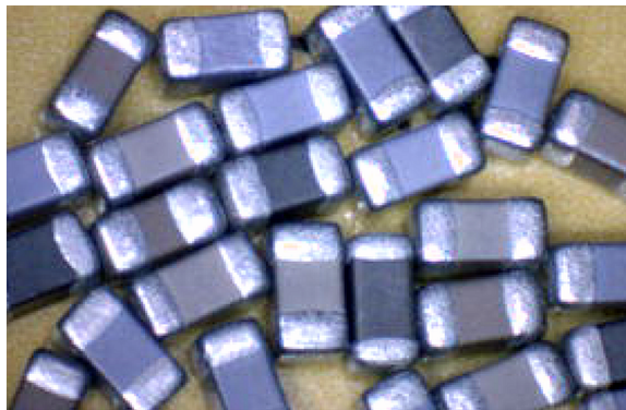
Figure 45 Multi-layer ceramic capacitors (MLCC chips) for SMD mounting
