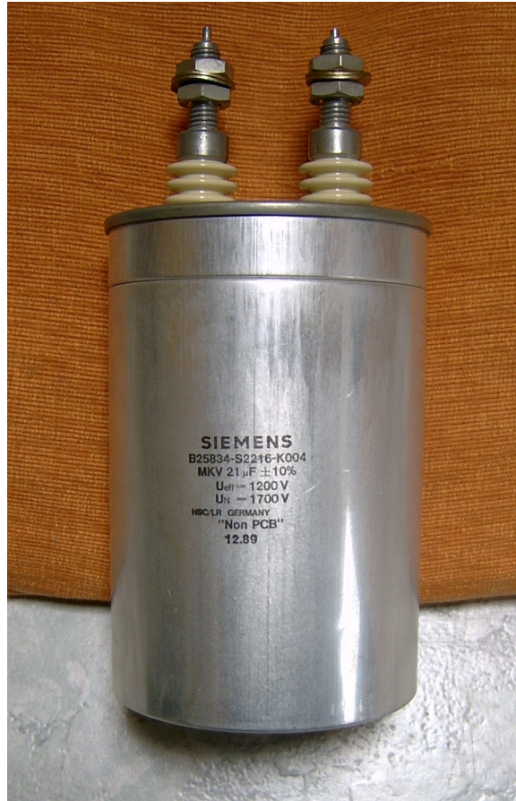
Figure 55 Power film capacitor for AC Power factor correction a (PFC), packaged in a cylindrical metal can
