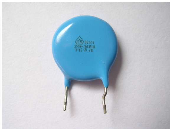
Figure 47 Ceramic EMI suppression capacitors for connection to the supply mains (safety capacitor)
