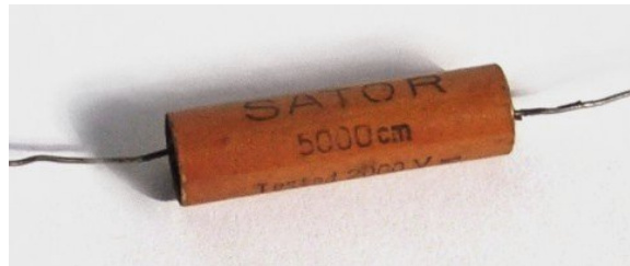
Figure 40 Wound metallized paper capacitor from the early 1930s in hardpaper case, capacitance value specified in "cm" in the cgs system a ; 5,000 cm corresponds to 28 nF
