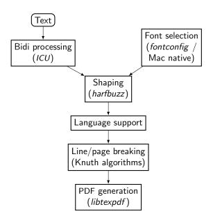
Figure 1: SILE's component parts
