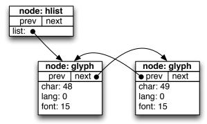
The *list* entry of the hlist (hbox) points to the *node list* starting with the digit 0. The idea for our second approach is to create a node list that represents the vertical bars and gaps (rule and kern nodes) and digits. We create a few more helper functions as well as the new main function:
