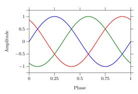
Figure 6: Three Phase Power
