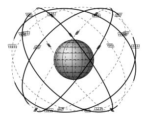
**Figure 11:** The U.S. GPS system. This view, looking directly at the equator, shows that the orbits never pass over the north or south poles. Each orbit has four satellites spaced 30 degrees, 105 degrees, 120 degrees, and 105 degrees apart.
