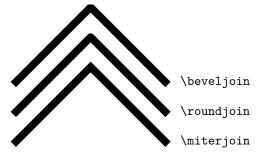
Figure 2: Join styles for line segments
