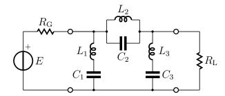
Figure 5: A band elimination filter
