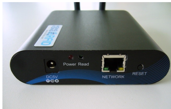
Fig. 1 Active RFID reader
