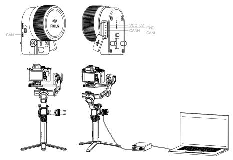
Users can also use the Ronin Series Accessories (RSA)/NATO ports of DJI RS 2 to directly connect with and control DJI RS 2. Below is an illustration of the RSA/NATO ports:
