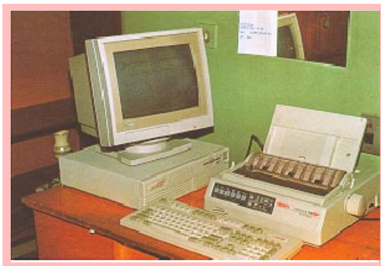
Figure 4 A typical monitoring and control unit (M&C) for remote control of an earth station from a Member's CNCT.
