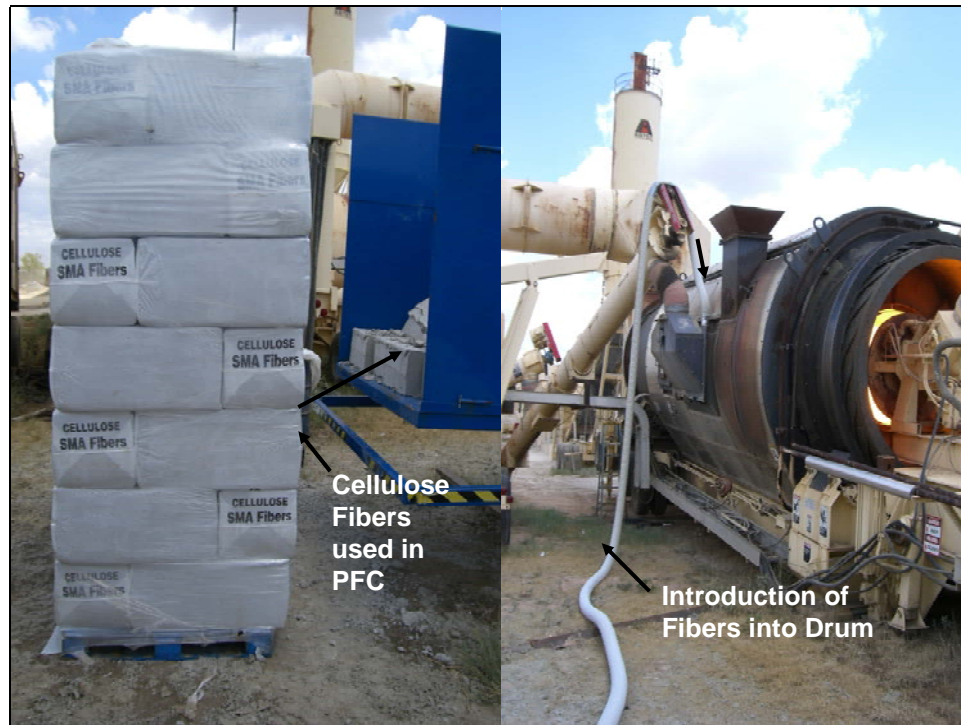
Figure 1. Introduction of Fibers into Drum on IH-30 Project in Paris District.
