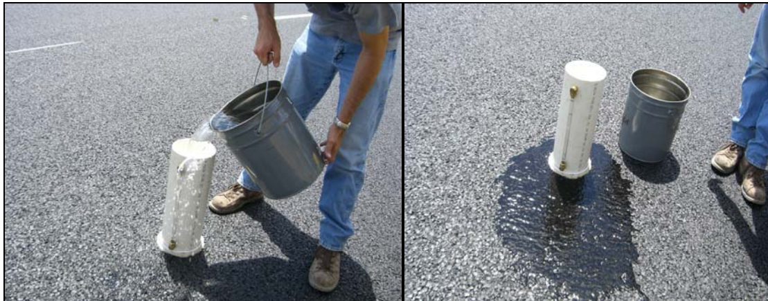
Figure 9. Test Method Tex-246-F, Field Water Flow Test.
