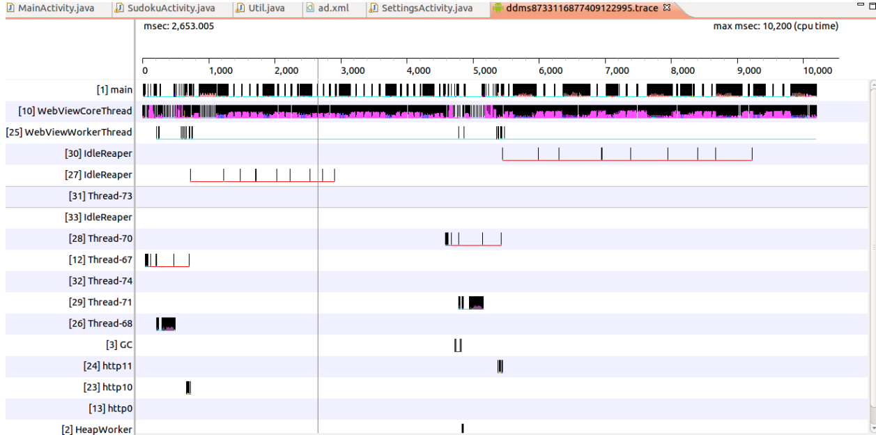
Fig. 3. A trace of the same App with anomalous Ads. Notice that main is doing much more work and there are other threads that are getting significant CPU time.
