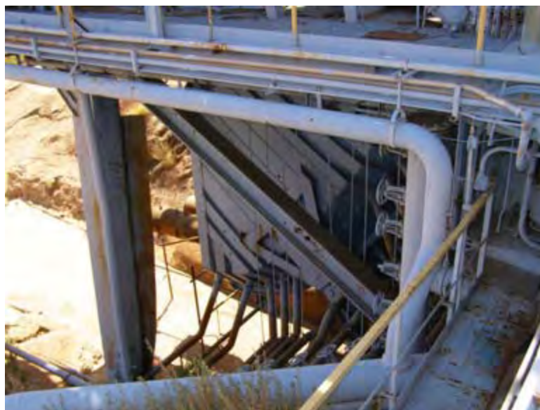
Photo 4.28. Bravo I Test Stand, flame deflector, camera facing east. (Source: Archaeological Consultants, Inc., 2007.)
