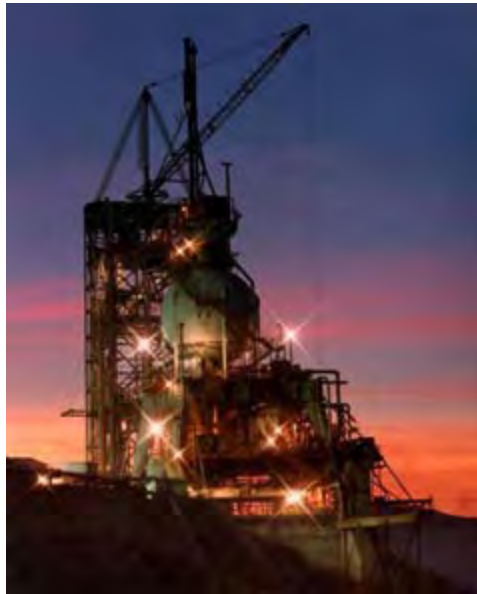
Photo 3.26. Preparations for SSME components test on Coca I (Test Stand A-3) at Santa Susana (NASA Area II), 20 December 1974.
