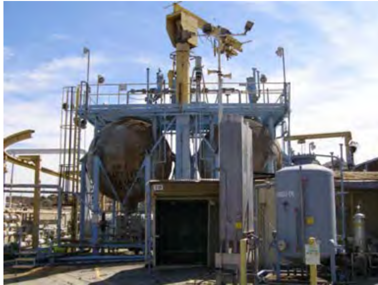
Photo 4.34. Bravo II Test Stand, Run tanks at north, RP-1 to left and LOX to right, camera facing southeast.
