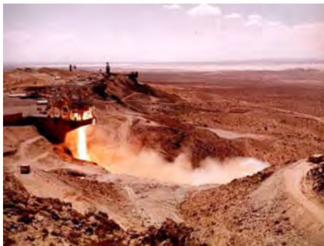
Photo 3.25. F-1 engine during hot firing at the Edwards Field Laboratory on Leuhman Ridge, Edwards Air Force Base, 11 August 1961.
