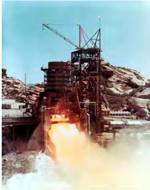
Photo 4.52. Coca I Test Stand, J-2 Five Engine Cluster hot fire test, August 1965, camera facing south.
