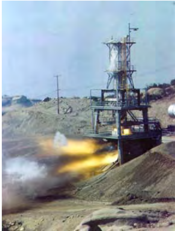
Photo 4.10. Alfa I Engine Hot Fire Test, date unknown, camera facing northeast. (Source: Boeing Company/Santa Susana Field Laboratory; Photo #133.)
