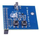
The "IR Remote Shield v1.0" product does not include drivers or interface software. Fortunately, there is an open source effort that provides the low level processing required to send and receive IR signals. LIRC or Linux Infrared Remote Control allows the IR signals to pass through the RPi. LIRC was first established in 1999 and has several distribution packages including one for the Raspberry Pi platform [2].
