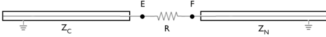
Figure B.2: The NCD cable with impedance Z_C connected to the resistive coupler of strength R , connected to the NCD counter with impedance Z_N . In the electronics model Z_C = 100 \Omega , R = 325 \Omega , and Z_N = 415 \Omega .
