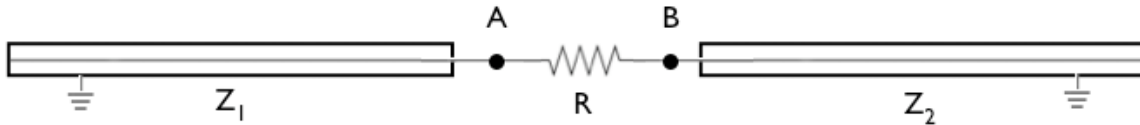
Figure B.1: Two transmission lines of impedances Z_1 and Z_2 , connected by a resistor of strength R .
