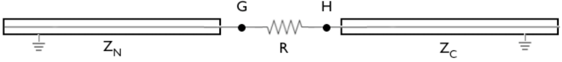
Figure B.3: The NCD counter with impedance Z_N connected to the resistive coupler of strength R , connected to the NCD cable with impedance Z_C . In the electronics model Z_C = 100 \Omega , R = 325 \Omega , and Z_N = 415 \Omega .
