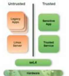
The microkernel therefore acts as a gatekeeper: enabling the separation of *trusted* and *untrusted* functions within the system.
