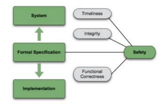
In addition, safety-critical systems often require *temporal integrity* – a guarantee that a less critical part of the system cannot affect the timeliness of a critical part.
