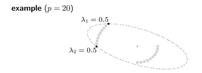
design uses two vectors, on boundary of ellipse defined by optimal  $\boldsymbol{W}$
